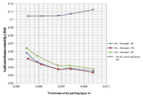
Fig. 6. Thermal conductivity coefficient  $\lambda$  (W·m<sup>-1</sup>·K<sup>-1</sup>) values of the samples with aerogel filling and air parting layer
