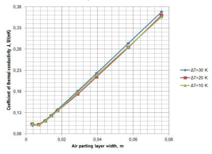
Fig. 4. Dependence of the coefficient of thermal conductivity on the air parting layer width for a horizontally positioned sample
