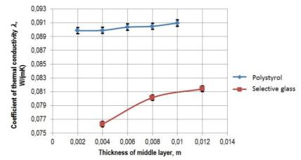
Fig. 8. Thermal conductivity coefficient  $\lambda$  (W·m<sup>-1</sup>·K<sup>-1</sup>) values for the samples with organic glass (polystyrol) and inorganic glass with selective coating in the middle layer
