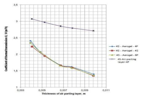
Fig. 7. Thermal transmission coefficient U (W·m<sup>-2</sup>·K<sup>-1</sup>) values of the samples with aerogel filling and air gap (calculated)
