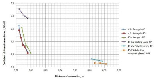
Fig. 10. Dependence of the thermal transmission coefficient  $U(W \cdot m^{-2} \cdot K^{-1})$  on sample thickness
