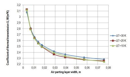
Fig. 5. Dependence of the thermal transmition coefficient on the width of the air separation layer, the values of the coefficients of thermal transmission are calculated
